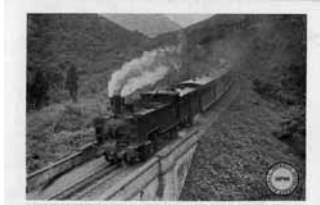
565 A TRAIN ON THE TRACK RUNNING UP A GRADE OF 1 IN 15 ...
